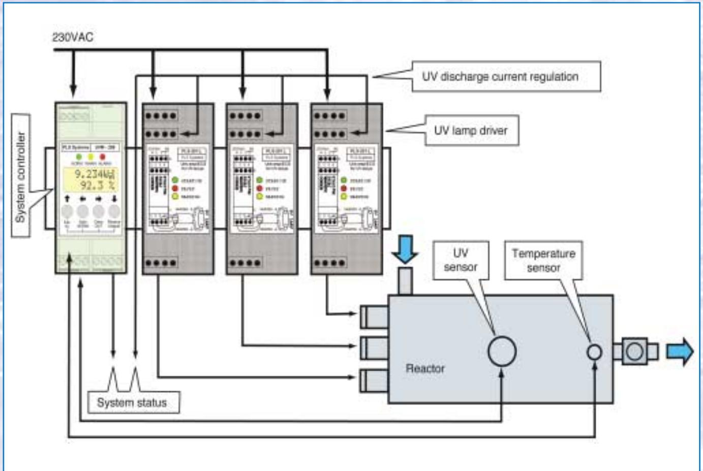
The patented Electronic Control Gear (ECG) is fitted with the most advanced controls to look after the performance of the Titanium AOP system.
