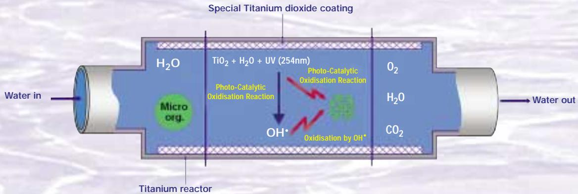
The Photo-Catalytic oxidation reaction has two effects. Primarily it will oxidise and destroy any microbe or pollutant present where the reaction occurs. In the case of the Titanium AOP this is the entire surface area of the reactor that is contact with the water. The second reaction oxidises water to generate a proliferation of Hydroxyl Radicals that in turn will also oxidise any microbe or pollutant present.
